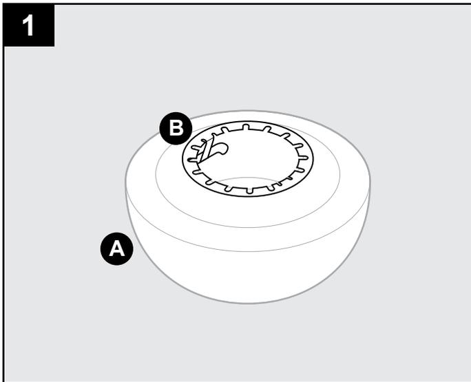
**Note:** Assure that the metal ring is attached inside the Fire Pot./
